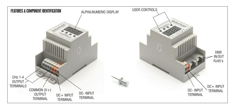
The QolorFLEX 4x5A DINrail RJ45 Dimmer can control a full 20A of LED tape spread over four channels of 5A each. It uses constant voltage technology which ensures consistent full range dimming that is especially important at low end light levels. The unit mounts to a standard hat section DINrail, and features two RJ45 connectors for DMX communication.
